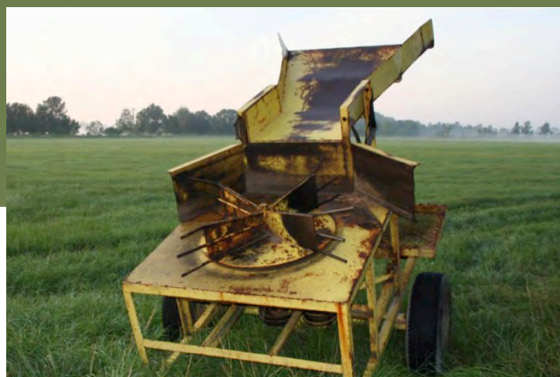
Figure 2. Square bales of bermudagrass tops are being scattered over a prepared seedbed (bottom left) using a ground-driven tops spreader (bottom right).
