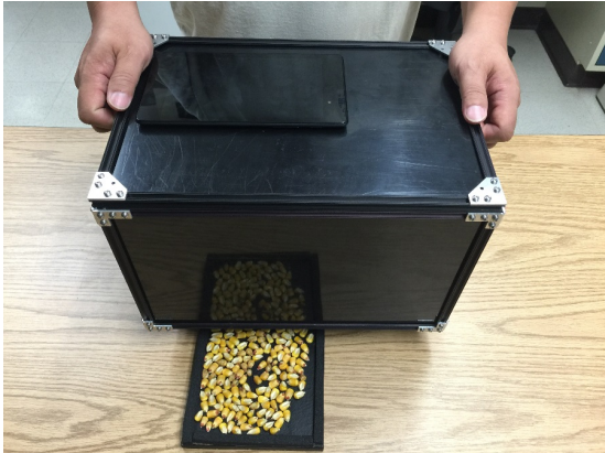
The aflatoxin detection prototype dubbed “aflabox” uses UV light to show the fluorescing of maize kernels contaminated with aflatoxin, which are visible in red.
