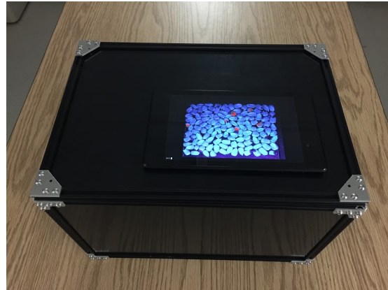
The aflatoxin detection prototype dubbed “aflabox” uses UV light to show the fluorescing of maize kernels contaminated with aflatoxin, which are visible in red.
