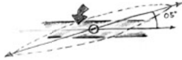
Figure 2A. Flat fan nozzles should be angled at approximately 5% from parallel to the boom. All nozzles should be turned the same direction. Graphics by Will Hampton.
