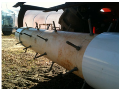
A close up of the bolts that punch holes for the transplants.
