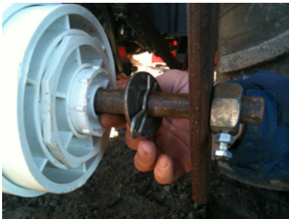
A close up of the RC Pinhead with the PVC bushings and steel rod axle.
