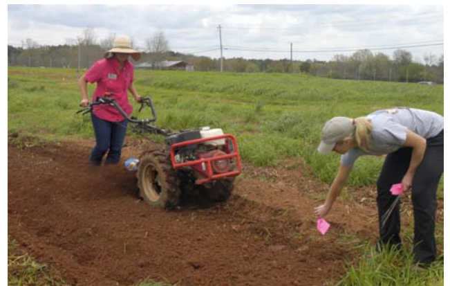
This BCS tiller is making a raised field bed with the rotary plow attachment. Operated by JoHanna Biang, UGArden Farm Manager.
