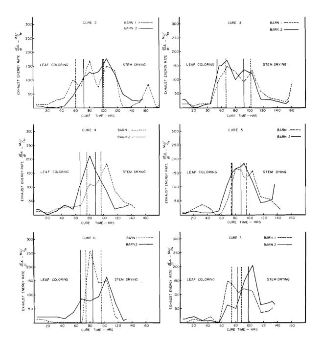
Figure 4. Exhaust energy rate for Barns 1 and 2, Cures 2-7 respectively.
