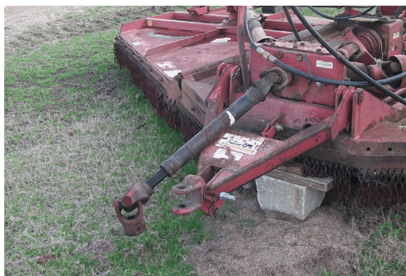
PTO driveline without safety guards.
